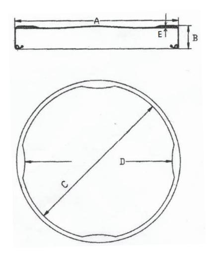
OUTSIDE DIAMETER: A:  $44.70 \pm 0.20$ mm HEIGHT OF CAP: B:  $8.80 \pm 0.20$ mm INNER DIAMETER: C:  $41.10 \pm 0.20$ mm
